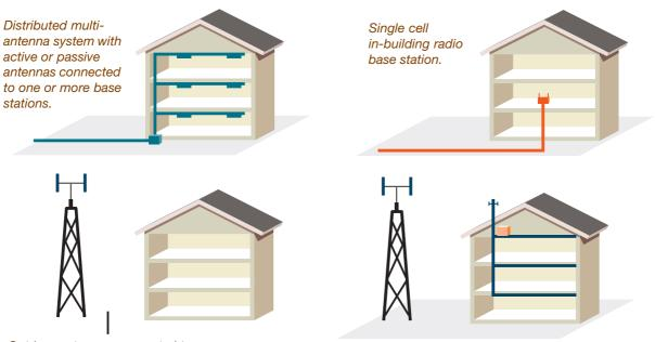
Outdoor antennas connected to macro or micro radio base stations, installed for instance on a mast or on a nearby building.
